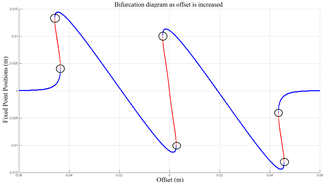
Figure 4.24: Bifurcation diagram for offset magnitudes of up to 6 cm with d = 3.93 cm. Solid curves are computed from the full model. Red indicates unstable fixed points, blue indicates stable fixed points. Saddle-node bifurcations are highlighted in circles.
